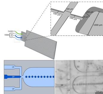
**Figure 1.** Schematic of the microfluidics chip. CP: continuous phase, DP: Dispersed phase.
