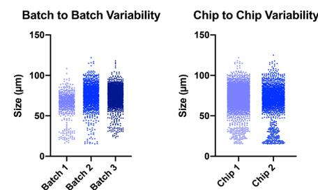
**Figure 6.** The microfluidic chips used to synthesize M2A2 showed little variability between batches and between chips. Differences between chips and between batches are not statistically significant.
