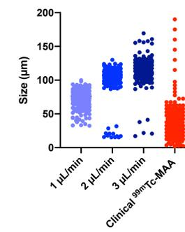
**Figure 5.** Altering the flow rate of the dispersed phase can lead to changes in the average particle diameter. The particle diameter of clinical <sup>99m</sup>Tc-MAA (adapted from Takagi *et al* is shown for comparison) [5]. Mean particle sizes were  $72.0 \pm 15.1$ ,  $105.6 \pm 14.7$ , and  $119.2 \pm 12.5$   $\mu\text{m}$  for DP flow rates of 1, 2, and 3  $\mu\text{L}/\text{min}$ , respectively. Clinical MAA had a mean particle size of  $32.7 \pm 17.8$   $\mu\text{m}$ .
